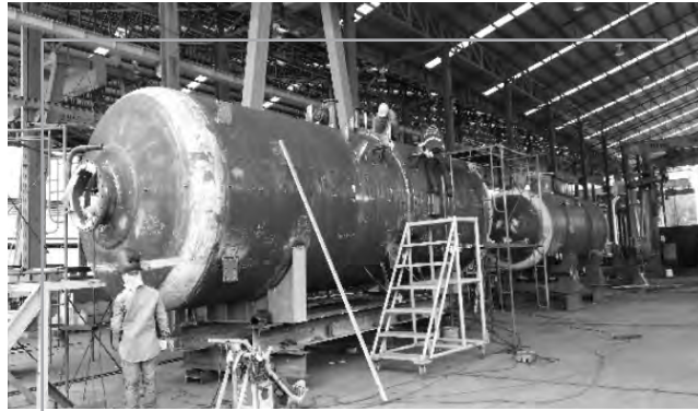
Heat Exchanger Fabrication
